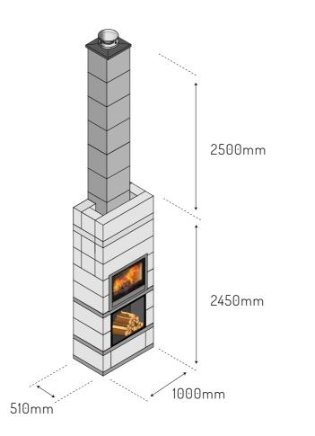
The Opus Scandfire system comes with a 2450mm high chimney breast chamber and 2500mm of chimney. Additional chimney sections are then added to the system as the project dictates. A choice of terminal is then added.
